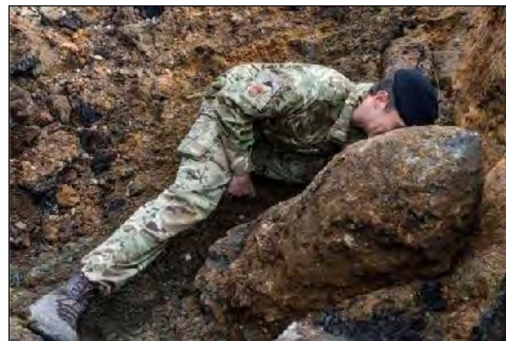
Top: J-curve Effect - Due to angle of entry, unexploded bombs would often end their trajectory at a lateral offset from point of entry, often ending up beneath adjacent extant structures/sites. The photograph above shows a 250kg unexploded bomb found in Bermondsey in 2015, pointing upwards, demonstrating 'J-curve'.
